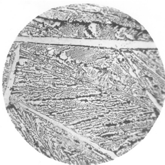
Fig. 78 The metallographic structure (100x) of white pig iron used in the Warring States period
