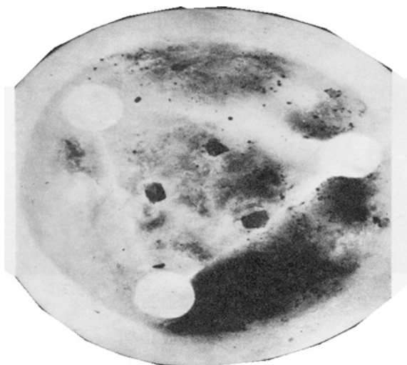
Fig. 20 Copper core support at the lower part of the belly of a Ding (pot) produced in Western Zhou Dynasty, excavated in Baoji, Shaanxi Province
