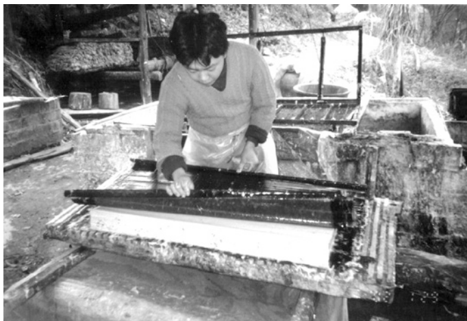
Fig. 14 Lift the curtain after putting the lift paper upside down on the paper stack
