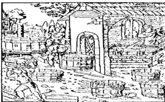
Fig. 49 Workshop for refining saltpeter and sulfur by Europeans in fifteenth century
