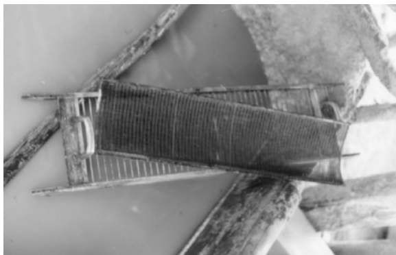
Fig. 12 Paper curtain and curtain support for papermaking in Chinese mainland
