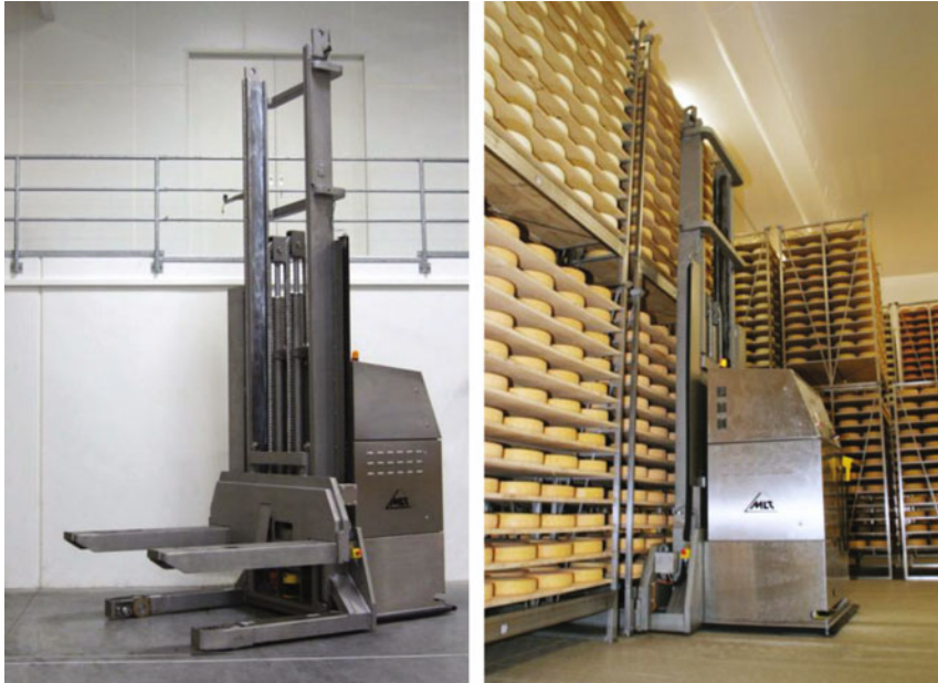
Fig. 2.43 The stainless-steel forklift carries 4.6 tons and reaches a lifting height of 3.8 m (Source MLR 2009)
