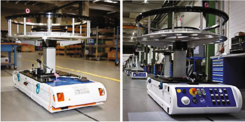
Fig. 2.73 The automated guided vehicle with rotating assembly mounting. ( front and rear view, Source Daum + Partner Maschinenbau GmbH, Aichstetten )
