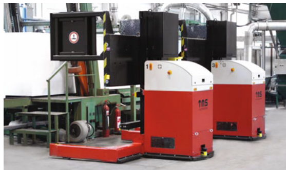
Fig. 2.44 The AGV with its enormous grippers for the delicate giants (Source DS 2007)
