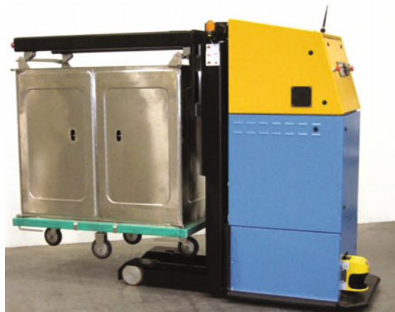
Fig. 2.50 A forklift AGV for frontal pickup of a roller container (Source MLR)
