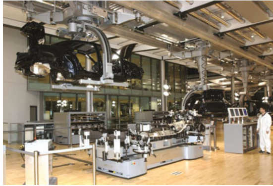
Fig. 2.14 The “wedding” station. The body approaches from above suspended from the overhead line, below in the foreground a AGV waits with the powertrain, in the back ground a goods-basket AGV drives past ( Source Volkswagen )
