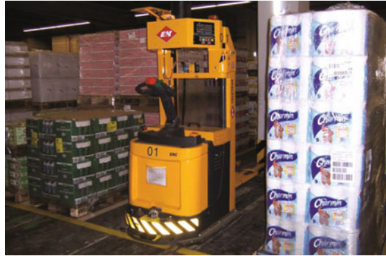
Fig. 2.39 A commissioning AGV, with optional manual operation ( Source E&K 2004 )
