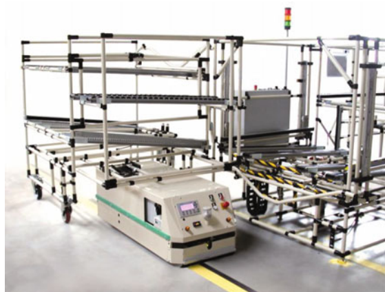
Fig. 2.26 Underride AGV tows the materials wagon with lateral gravity transfer system based on the Minomi principle (Source CREFORM 2009)
