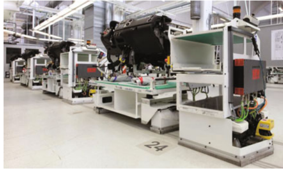
Fig. 2.25 A combination of tractor and assembly AGVs (Source SEW 2010)
