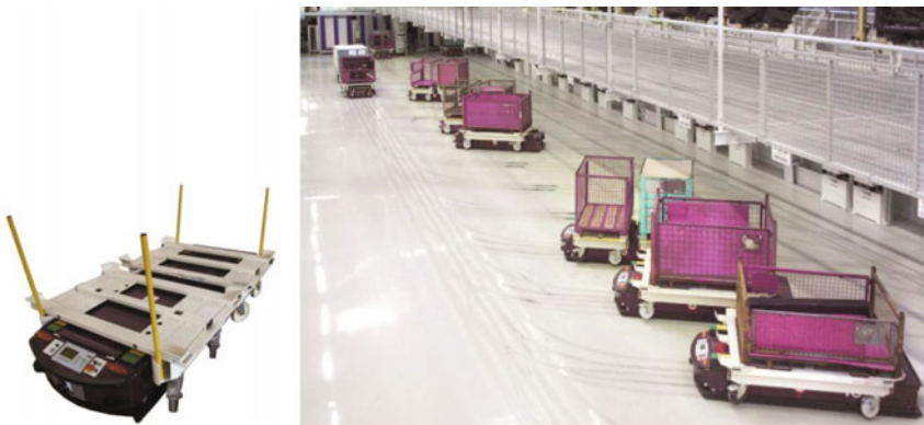
Fig. 2.19 Left Detailed view of a vehicle with two sequencer frames. Right Battery loading station for the NiCd batteries ( Source DS )
