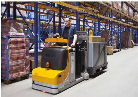
Fig. 2.80 Manual riding: two contacts in the floor place as well as the two SAFE balls must be engaged while driving ( Source DS 2012)
