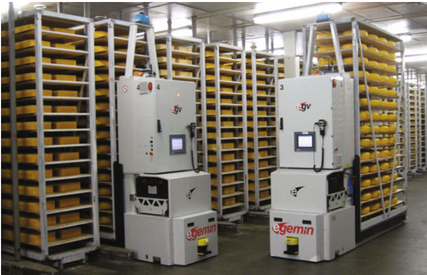
Fig. 2.42 Two vehicles handling cheese in the aging warehouse (Source Egemin 2008)
