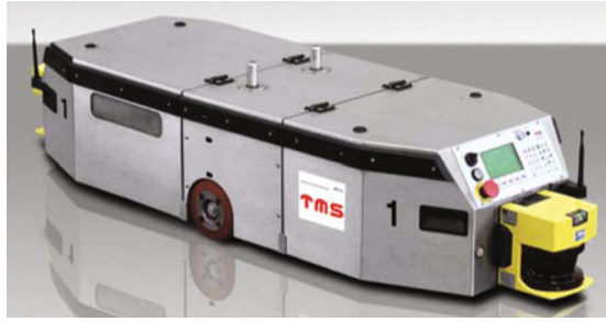
Fig. 2.51 Underride AGV with thorn pickup for towing roller containers ( Source DS)
