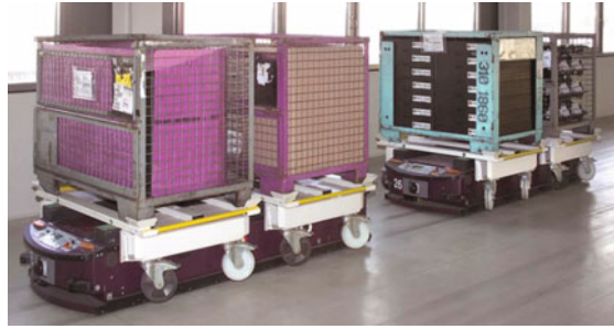
Fig. 2.16 Underride AGVs with small trolleys for pallet cages (Source DS 2006)
