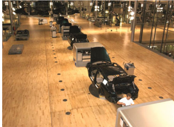
Fig. 2.13 Vies of the assembly line. A conveyor set in the floor snakes its way through the assembly area (Source Volkswagen)
