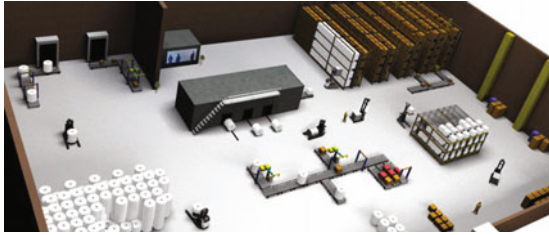
Fig. 2.1 An AGVS connects various processes in paper roll handling (Diagram, Source Rocla)
