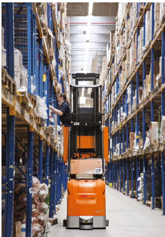
Fig. 2.81 Manual commissioning on the 2nd and 3rd storage level ( Source DS 2012)
