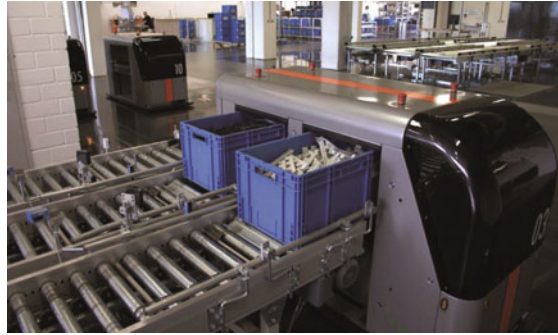
Fig. 2.35 Material delivery in the assembly area (Source FROG)
