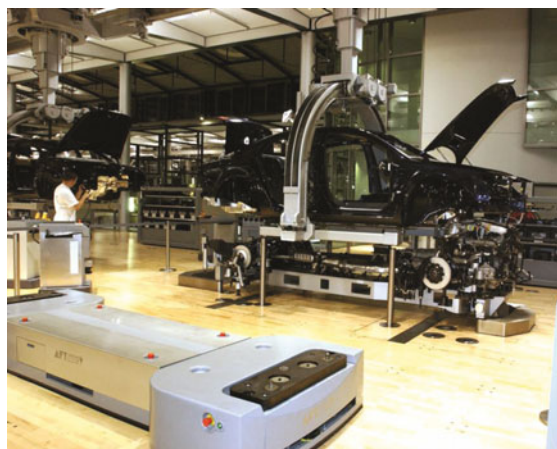
Fig. 2.15 Once again the wedding station: in the foreground and empty AGV leaves, behind it the “wedding”, powertrain from below, body from above ( Source Volkswagen )
