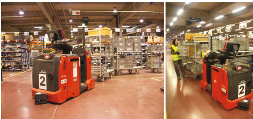
Fig. 2.28 AGV as towing tractor: rebuilt Linde tractor (Source E&K)
