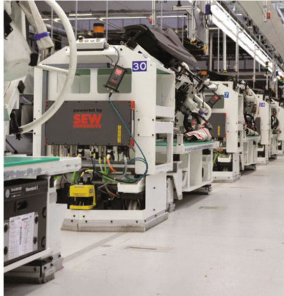
Fig. 2.24 Thirty AGVs in a simple assembly layout for cockpits (Source SEW 2010)
