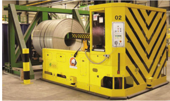
Fig. 2.48 Coil transfer from the coil lifter to the turnstile (Source FROG 2005)
