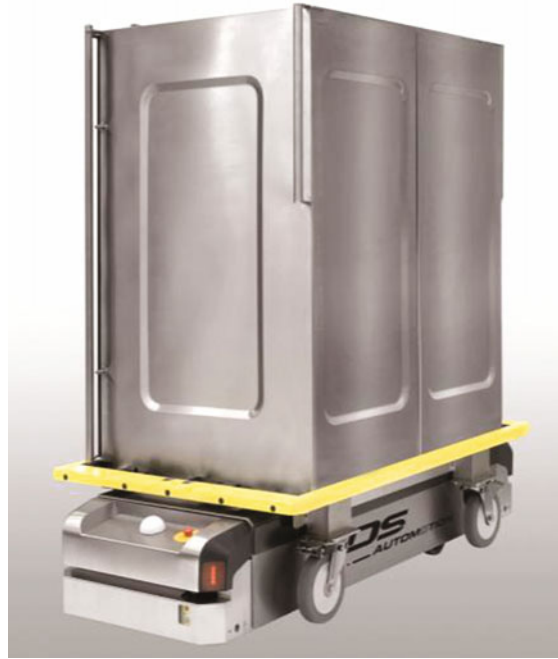
Fig. 2.53 A AGV carries a roller container. The vehicles have a maximum payload of 500 kg ( Source DS 2009 )
