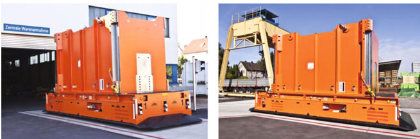
Fig. 2.74 Automated guided heavy load transport crosses the outside area, carrying loads of up to 63 tons (Source MLR 2012)
