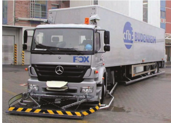
Fig. 2.11 Safety features on an outdoor AGV ( Source Götting )
