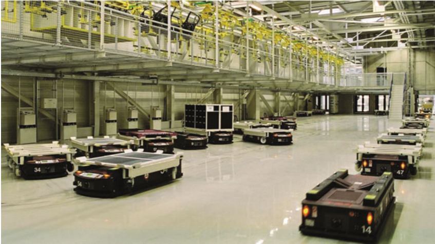
Fig. 2.17 The AGV with oversized roller carts for picking up large containers ( Source DS )
