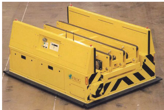
Fig. 2.49 AGV for disposable pallets with trimmed sheet metal up to six tons in weight (Source FROG 2005)
