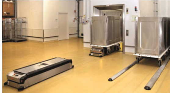
Fig. 2.54 Waiting for the elevator. The lifting and depositing positions directly on the elevator make it possible to dispatch roller containers (Source DS 2009)
