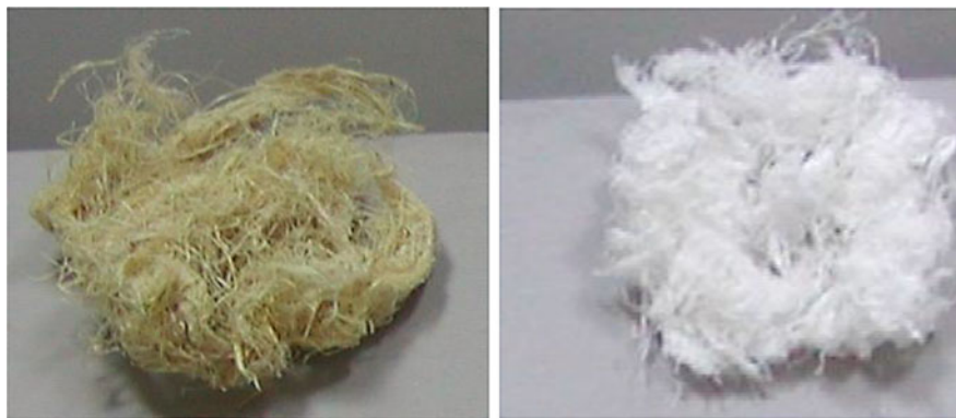
Fig. 2.1 Fibers extracted from cornhusks before ( left ) and after bleaching ( right ) to a CIE WI of 74
