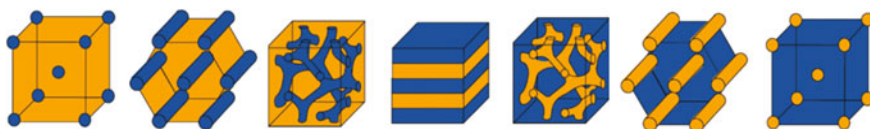
Fig. 2.4 Different morphologies of block copolymers. From left to right an increasing fraction of the blue block , resulting in spherical, cylindrical, gyroid, lamellar, and the inverse structures , respectively. Adapted with the permission from Ref. [33]. Copyright 2010 American Chemical Society
