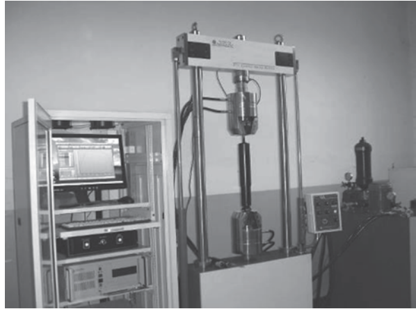
Fig. 2.2 Experimental setup for testing shock absorber. (Reprinted from ref. [11], Copyright 2013, with kind permission from Maxwell Scientific organization)
