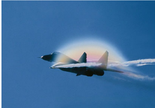
Fig. 2.4 Coexistence of wingtip vortices and supersonic waves around a fighter flying at nearly sound speed. Courtesy of http://www.sky-flash.com/EJ.v.Koningsveld
