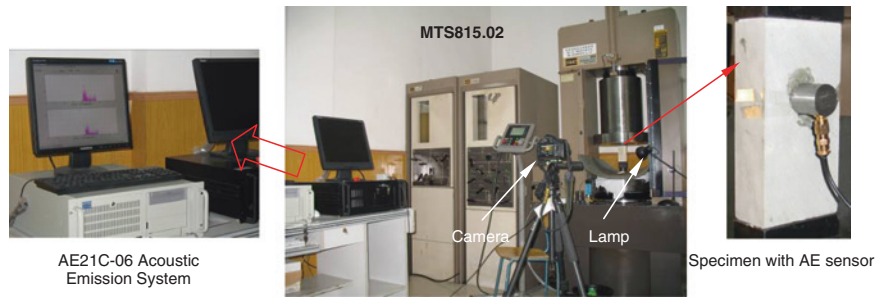
Fig. 2.4 MTS815.02 rock mechanics servo-controlled testing system and AE21C-06 acoustic emission system, in which the camera and lamp were used to record clearly the crack coalescence process of sandstone (with kind permission of Springer Publisher)
