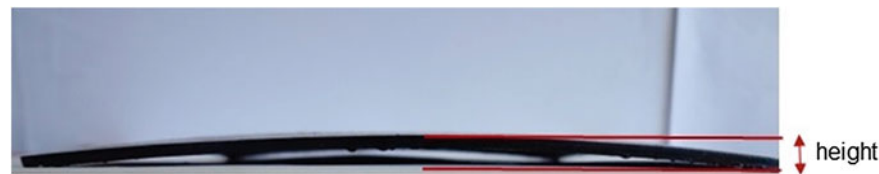
Fig. 25 Dome shaped specimen after laser forming. The horizontal red lines show the dome height measured from the base to the top most point at the center of the specimen
