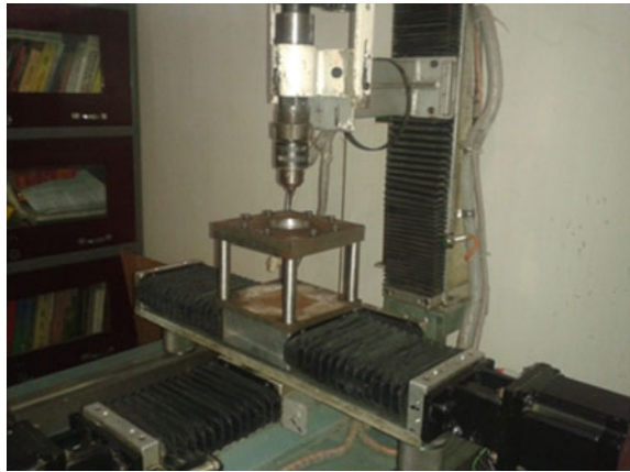
Fig. 18 Single-point incremental forming machine
