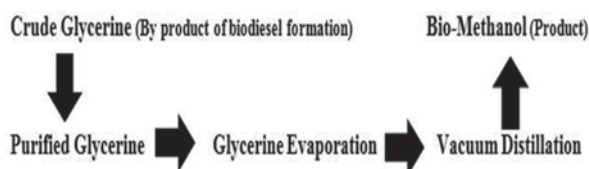
Fig. 2.3 Methanol production using Bio-MCN process, the crude glycerin processing leads to bio methanol production
