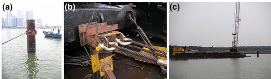
Fig. 20 Load testing of mooring piles. a Pull cable attached to pile. b Pull cable attached to winch onboard barge and c pull load test set-up with barge
