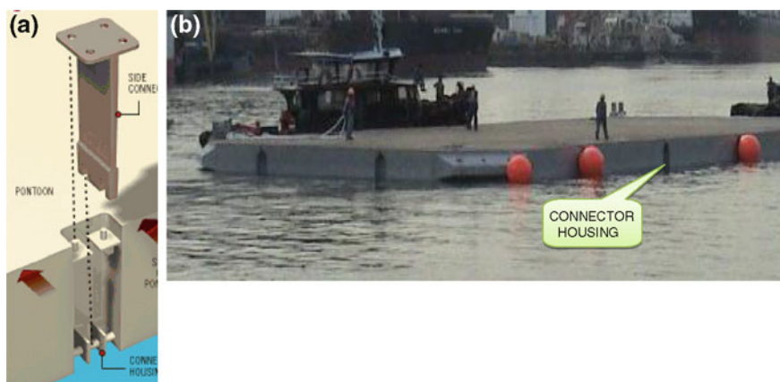
Fig. 7 Joining the pontoons using the side connector
