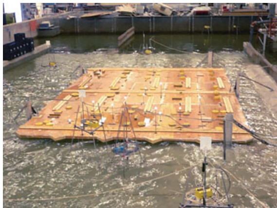
Fig. 17 Hydrodynamic model test
