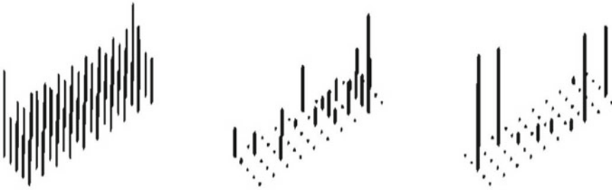
Fig. 2.3 Illustration of different degrees of sparseness. According to (2.7), the S_{\mathbf{X}} values corresponding to the three 2-D signals (from left to right) are 0.1, 0.5, 0.9, respectively
