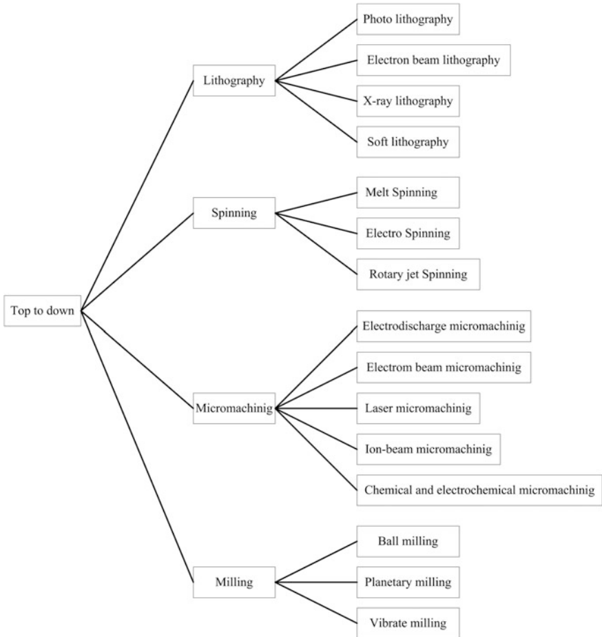
Fig. 2.9 Classification of the common top-down methods for nanostructural material synthesis or production
