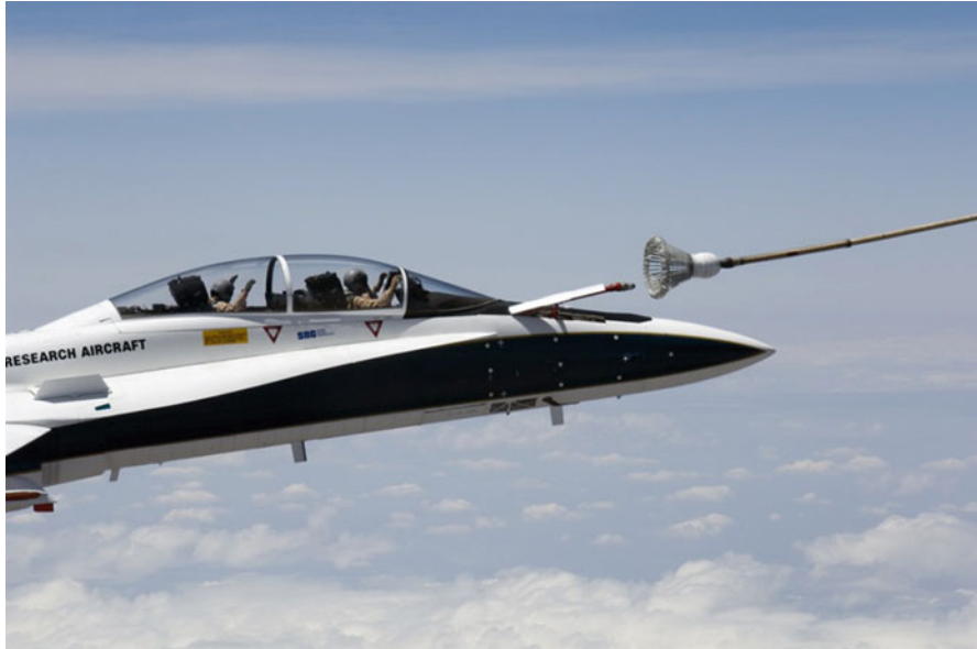
Fig. 2.5 Aerial refueling using the hose-and-drogue system
