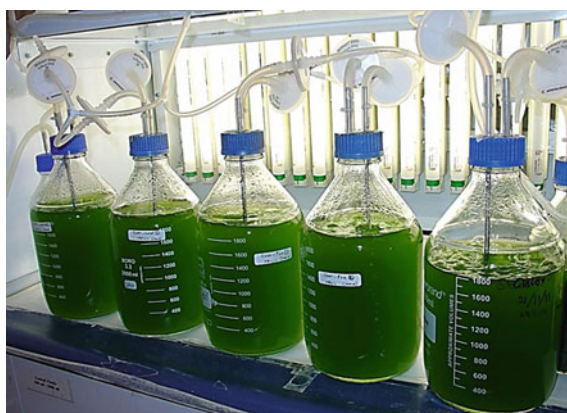
Fig. 6 An early monoseptic stage of production of an algal inoculum for a small raceway
