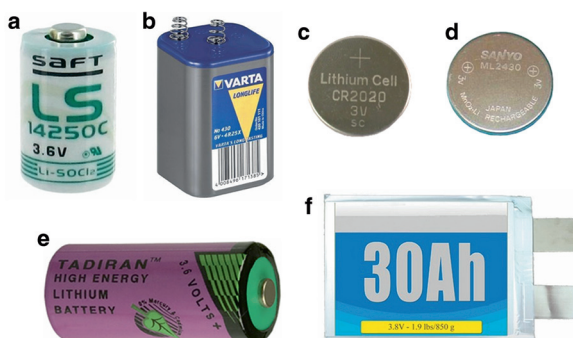
Fig. 2.13 Various battery configurations. (a) LS14250- cylindrical Li// \text{SOCl}_2 battery, (b) 4R25-prismatic (container) cell, (c–d) CR2020 Li- \text{MnO}_2 coin cells, (e) AA-type Li-ion cylindrical (1.5 Ah, 3.6 V, 12.4 g) cell, and (f) 30-Ah pouch ( \text{LiMn}_2\text{O}_4 -type, 3.8 V, 850 g) cell
