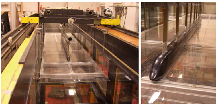
Fig. 1 A train model mounted on the moving model rig with the installed ground plate in the water towing tank at DLR Göttingen
