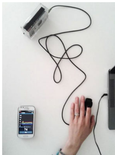
Fig. 4 Image of the CardioAlert prototype. On top left , the heart rate recorder that receives the changes in the hemoglobin detected by a led sensor connected to an individual’s finger. This signal is filtered, amplified and elaborated to obtain the heart rate by using an Arduino microcontroller. On bottom left , is the smartphone which receives the data from the microcontroller by a bluetooth connection
