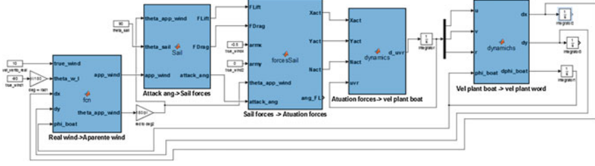
Fig. 7 Complete simulation model of the hybrid ASV developed in Simulink
