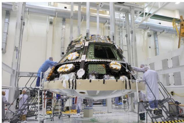
Fig. 2.15 Engineers completing the installation of the heat shield on NASA's Orion spacecraft. The Avcoat ablative material is covered with a silver reflective tape that protects it from the extreme cold temperatures of space. The heat shield has been shown able to protect the Orion crew from temperatures in the order of 2800 °C during re-entry and ocean splashdown (courtesy NASA)
