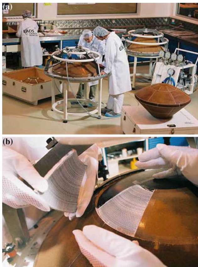
Fig. 2.24 The Beagle 2 Mars entry probe fitted with cork TPS. a Front-shield and back cover inspection in assembly workshop. b Front-shield tile being bonded—prior to packing in bio bags and sterilization treatment
