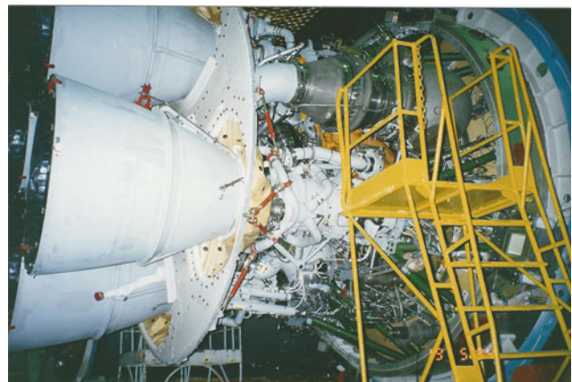
Fig. 2.10 Installation of Zenit first stage kerosene–LO 2 engine
