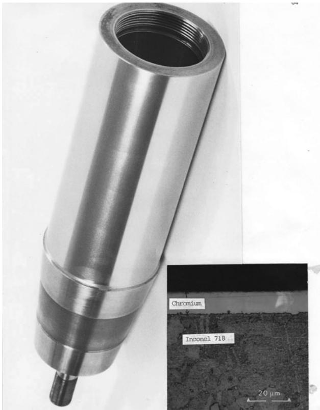
Fig. 2.5 Example of 300 mm long Spacelab pallet trunnion—machined from Inconel 718 and hard chromium plated. The insert shows plating to be 10 \mu\text{m} thick and well bonded to the etched substrate
