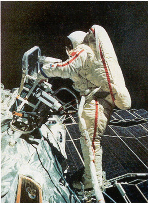
Fig. 2.29 Universal hand-held 3 kW manual EB gun used on Mir space station ( source from 1999, Avtomaticheskaya Svarka , 10)
