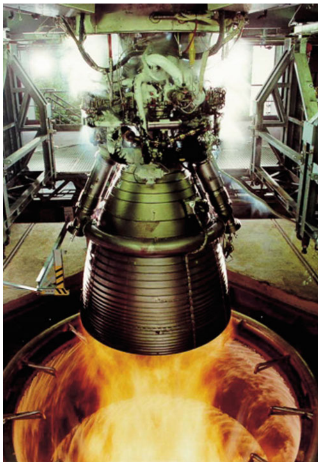
Fig. 2.13 Test firing of the Vulcain-2 engine (courtesy of SNECMA, France). The nozzle exit diameter is 2.5 m. Liquid hydrogen fuel is used to cool the engine, flowing through a jacket surrounding the thrust chamber. The heat absorbed this way is necessary in prolonged firings and enhances the initial energy content of the LOX and LH2 propellants prior to injection into the combustion chamber where the highly exothermic reaction produces steam ( 2\text{H}_2 + \text{O}_2 \rightarrow 2\text{H}_2\text{O} ) and more than 1000 kN of thrust. The nozzle supports rectangular tubes made from Inconel ® and welded together to form a helical structure through which the hydrogen coolant flows (Suslov et al. 2010)
