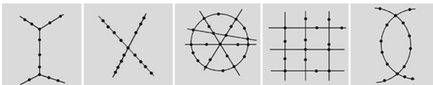
Fig. 2.18 Examples of rail network structures: diametrical with branching (X-system), radial (cross-system), circle-radial system, intermeshed-system and air-bladder system
