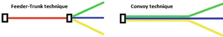
Fig. 2.26 Two techniques for network planning: “Feeder-Trunk technique” and “Convoy technique” (HiTrans 2)
