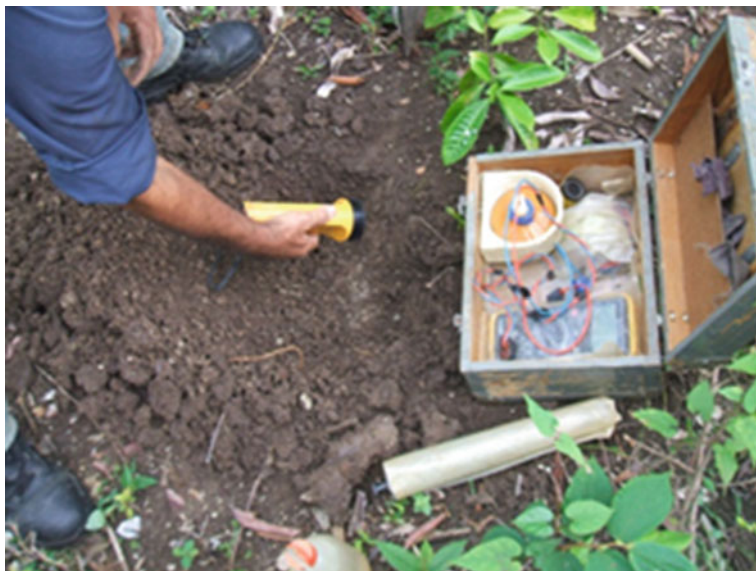
Fig. 2.2 Measurement of the Magnetic Susceptibility in soils
