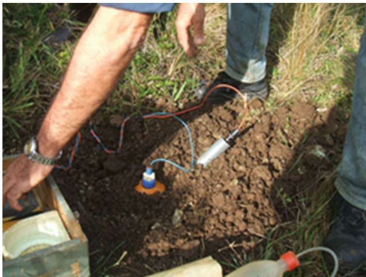
Fig. 2.1 Measurement of Redox Potential in soils
