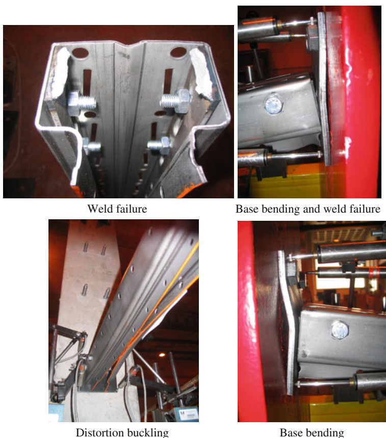
Fig. 2.41 Collapse modes for specimens bent in cross-aisle direction with bolts in tension
