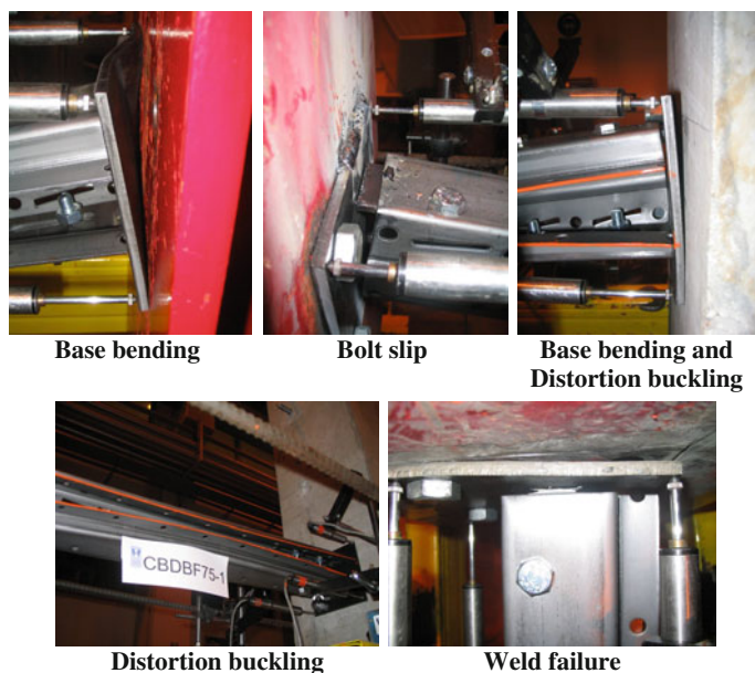
Fig. 2.48 Collapse modes for specimens under monotonic bending in down-aisle direction
