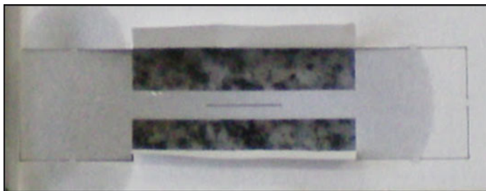
Fig. 2.14 Prototype device for two electrode measurement
