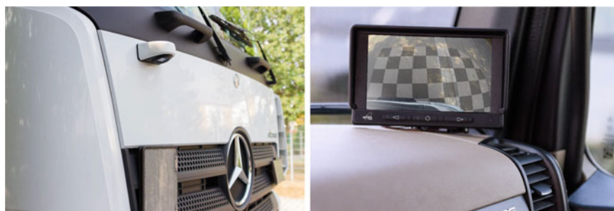
Fig. 12 Class VI Camera Monitor System (© MEKRA Lang GmbH & Co. KG)
