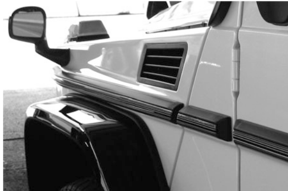
Fig. 15 Fender mirror of Mercedes-Benz G-Class (G463), right hand drive for Japan (© Daimler AG)
