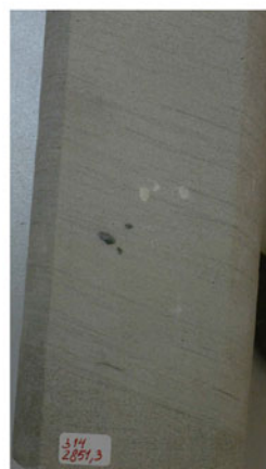
C. No stain in micro-porous Jurassic tidal flat sandstone, Russia. Porosity 7-10%, permeability < 1 md. Even on a 100 meter column of oil, this rock acts like a seal
