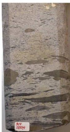
B. Spotty stain in low permeability Jurassic tidal channel sandstone, Russia. Porosity 10-15%, permeability 5-30 md
