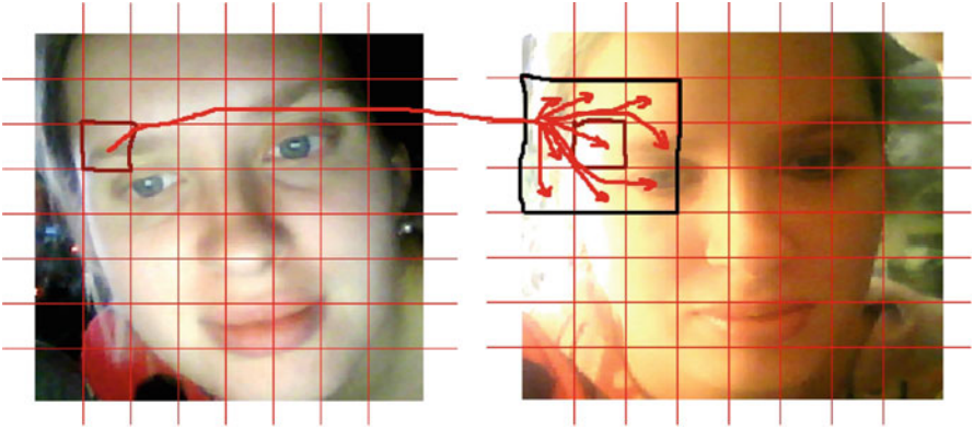
Fig. 2.1 The typical alignment of the segment of the input image ( left ) in the neighborhood of the corresponding segment in a reference image ( right )
