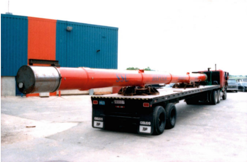
Fig. 2.3 SSC 50 mm collider dipole complete magnet
