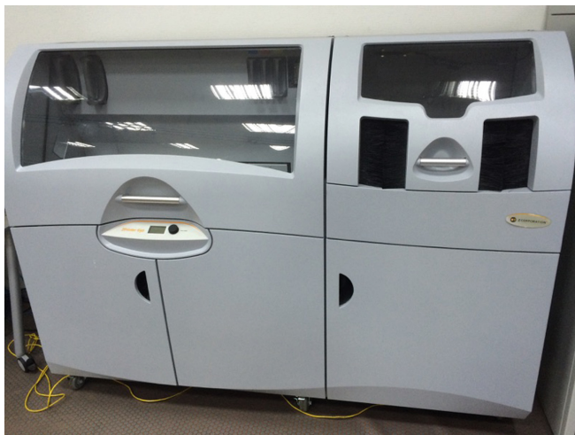
Fig. 6 3D printing system Zprinter 650 used for prototyping of the model S8 (Q-4)
