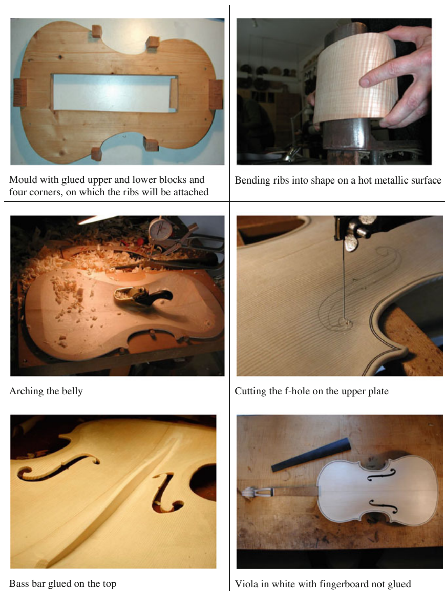
Fig. 2.40 Some aspects of violin building (Photos violin master HH Uilderks—Lübeck Germany. http://www.geigenbauonline.com/violinmaking-New-Construction.html . Access 10 April 2014)
