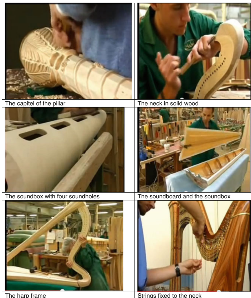
Fig. 2.44 Some operations for the technology of the concert harp (Photos Salvi Harps http://salviharpsinc.com . Access 7 October 2015)
