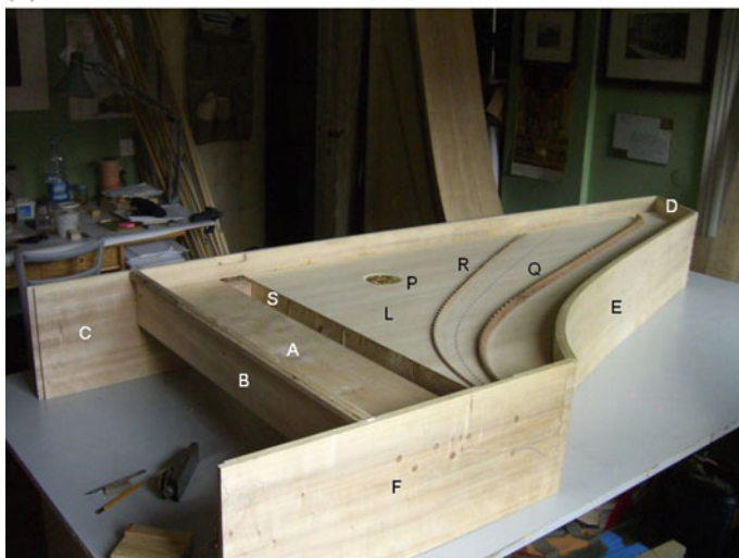
Fig. 2.50 Structural elements of a replica of a 18th century French harpsichord made by Taskin and recently built by Marco Brighenti—harpsichord maker in Parma— http://www.brighenti-harpsichords.com/images/foto/Taskin_soundb_01.jpg . Access 4 August 2014). Legend a internal structure; b upper view: A westplank; B nameboard; C spine; D tail; E bentside; F cheek; G upper bally rail; H lower belly rail; I lower frame; J arch; K liners; H lower frame; L soundboard; M 4' hitchpin rail; N cut-of-bar; O soundboard bars; P rosette; a Internal structure. A Sommier, B Barre de nom, C Echine, D Pointe, E Eclisse courbe, F Joue, G Contre-sommier, H Masse, I Barres de fond, J Arcs-boutants, K Contre-éclisses; L Table d'harmonie; M Boudin; N Grande barre; O Petites barres; P Rosace. b Upper view. A Sommier; B Barre de nom; C Echine; D Pointe; E Eclisse courbe; F Joue; L Table d'harmonie; P Rosace; Q Chevalet du 8 pieds; R Chevalet du 4 pieds; S Fosse. A -wrestplank, E -rib; F - L -soundboard Q -bridge 8'; R bridge 4'
