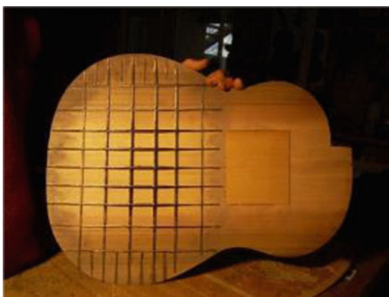
Fig. 2.58 Internal frame and rectangular lattice of a concert guitar made by Caldersmith ( http://www.caldersmithguitars.com/concert.php . Access 7 February 2014)
