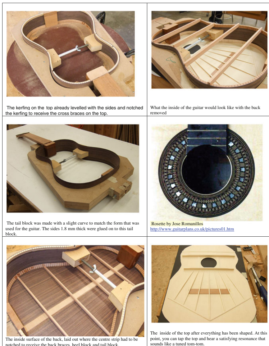
Fig. 2.41 Main operation for building of a concert classical guitar (Photos http://lumberjocks.com/kem/blog/6089 . Access 8 April 2014)
