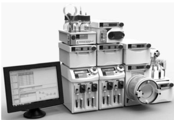
Fig. 2.3 SYRRIS System Asia™ 230 modular system
