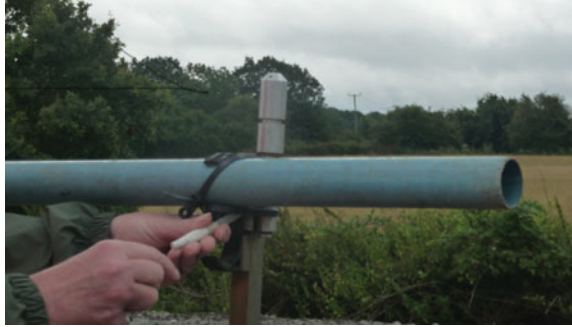
Fig. 2.16 The pressure probe and mounting used for the Uffington experiments
