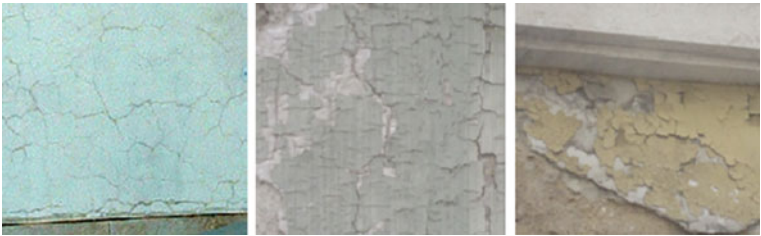
Fig. 2.10 Cracking defects in painted surfaces (data sourced from Chai 2011)
