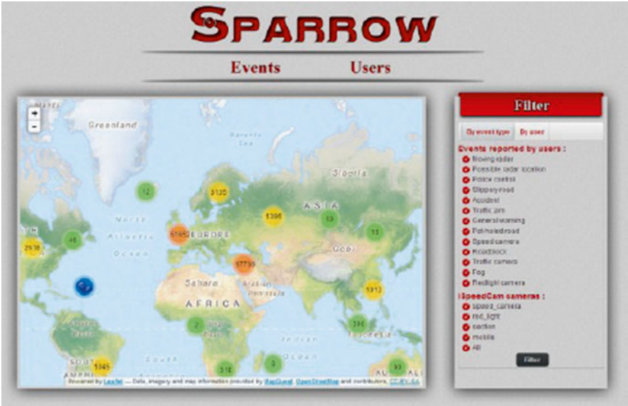
Fig. 2.7 Map view, data clustering, filtering (administration user interface). The Sparrow software incorporates a web-based administration user interface, which permits the system administrator to analyze all the available traffic incidents and cameras on a map. The events are clustered with an aim large quantities of data to be correctly represented (Adopted from [48])
