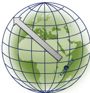
Fig. 2.3 Surfaces of position for range measurements
