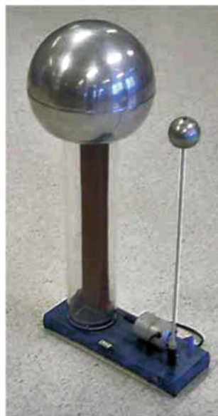
Fig. 1.5 The Van de Graaff generator and its working mechanism. Reproduced from Ref. [17]
