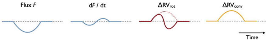
Fig. 2.10 The FF' method for a spot crossing the stellar disc. The RV variations induced by flux blocking ( \Delta RV_{\text{rot}} ) and suppression of the convective blueshift ( \Delta RV_{\text{conv}} ) are proportional to F dF/dt and F^2 , respectively
