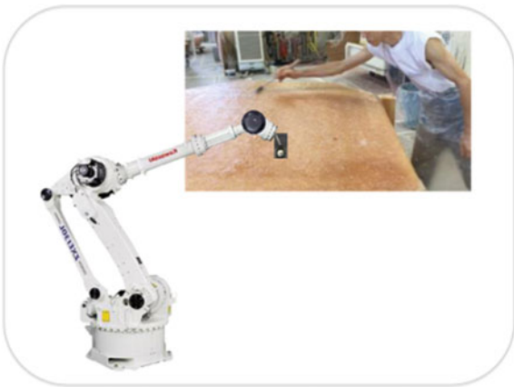
Fig. 12 Robots with advanced skills in hand lay-up
