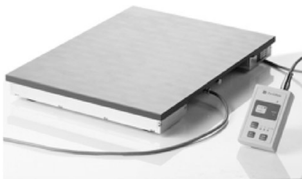
Fig. 5 Reaction force measuring device
