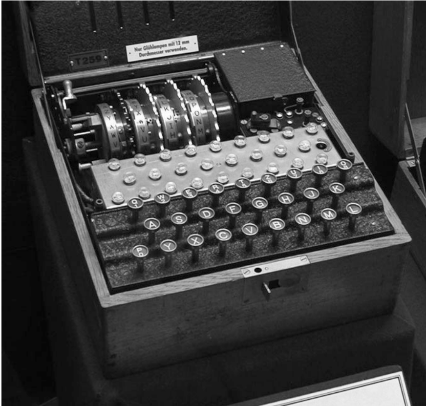
Fig. 1.1 Four-rotor Enigma machine
