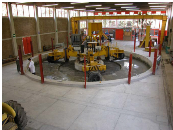
Fig. 3 Image of the slabs with crushed tire rubber in the circular track
