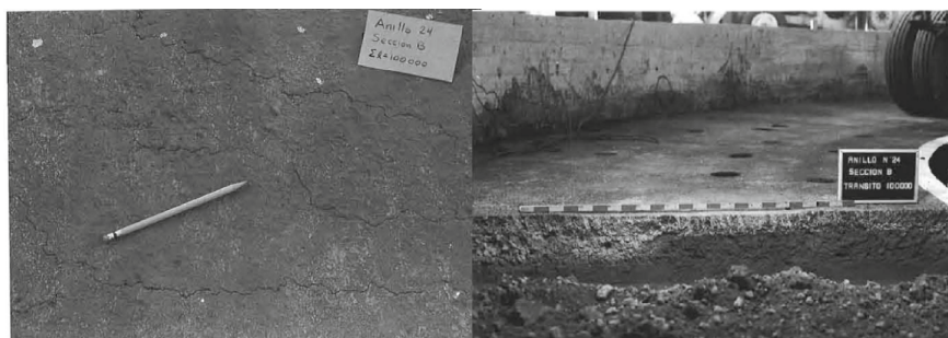
Fig. 2 Pavement section after the test at the circular track
