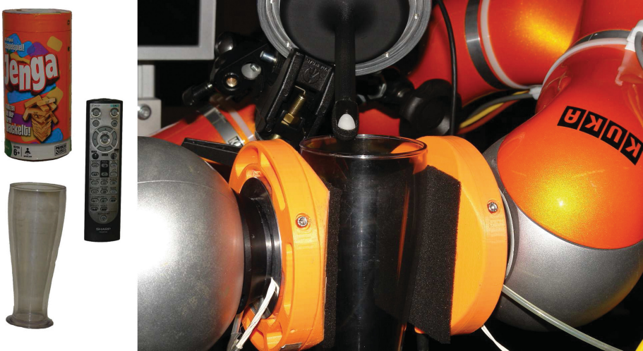
Fig. 1. Objects used for the evaluation and experimental setup for data recording. Two KUKA LWR robots with attached tactile sensors (light orange) holding a glass. The fingertip shaped sensor touching the glass from above is used to detect the onset of slippage for data labeling purposes. (Color figure online)
