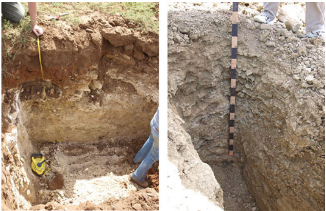
Fig. 2.1 Soil profiles showing two different degrees of development. Shallow Calcaric Cambisol ( left ) and deeper Vertic soil ( right )
