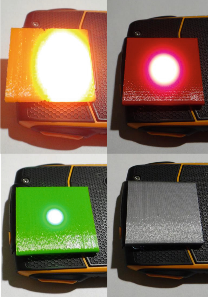
Fig. 5. Illustration of semi-transparency of some 3D prints for different types of PLA filaments illuminated from back side (orange, red, green and non-transparent gray). (Color figure online)
