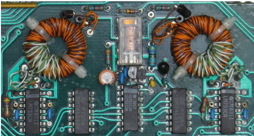
Fig. 3. Line isolation transformers. Detail from Fig. 1d showing hand-wound toroidal line isolation transformers and associated components
