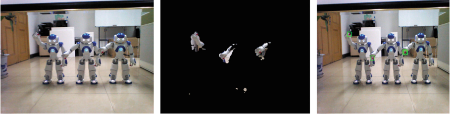
Fig. 3. Visual inputs and motion detection for robots mirror self-recognition
