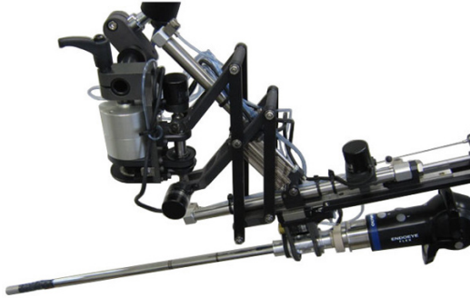
Figure 2.35: The pneumatic endoscope holder by Tadano et al. (Source: [145]).
