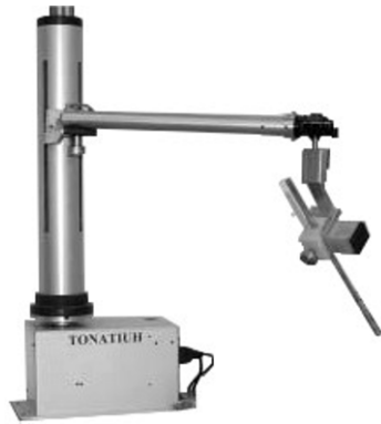
(a) The Tonatiuh II endoscope holder (Source: [137]).
