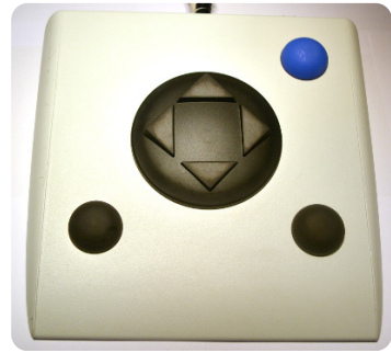
(b) ViKY control interfaces: Discrete voice commands and a foot pedal for continuous control
