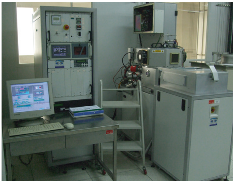
Fig. 2.2 The ICP equipment applied in the DRIE process
