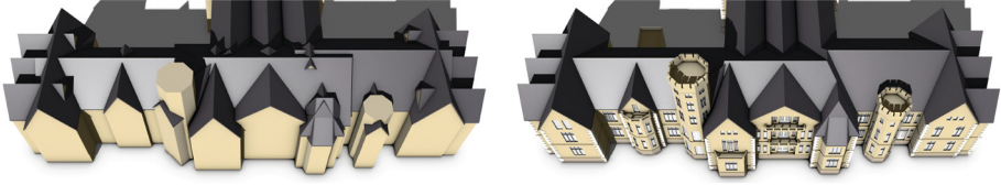
Fig. 1. Modeling a building by parametrizable parts greatly reduces the necessary effort. A simple union of parts might lead to undesirable results (left). Therefore, we introduce automatic roof trimming for solid building primitives. The resulting model can be further refined using existing procedural approaches (right).
