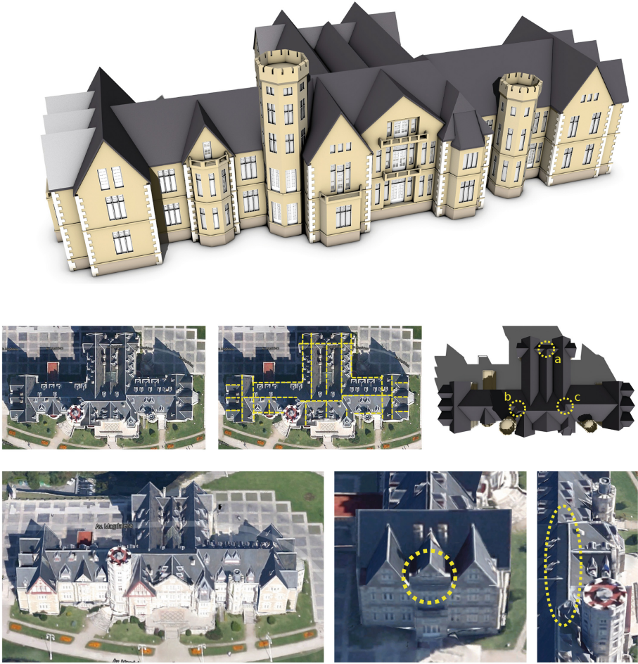
Fig. 21. Model of the Magdalena palace in Santander, Spain (as in the teaser - Fig. 1). The modeling process was done with aerial images (middle left, middle middle) as in Fig. 19. The detail of the model is increased with existing procedural approaches. Here we used a conventional shape grammar approach for modeling the facades (top). The model has three cases where roof topology changes because of a specified trimming (middle right - marked with yellow circles). (a) is the top row case from Fig. 9, (b) is the middle row case from Fig. 9, and (c) is a complex case where five solids with different trimming specifications are involved. The bottom row shows the 3D model in Google maps on the left. Again the constraints of planarity of roof faces and straightness of edges are not satisfied. Two additional regions with wrong geometry are emphasized in yellow circles. Aerial images: Map data ©2015 Google, basado en BCN IGN España.
