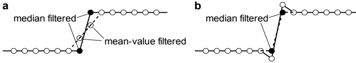
Fig. 2.5. Effects of filters with neighborhood \mathcal{N}_2^{(2)} (width 3) a Median filter and mean-value filter at a flat amplitude discontinuity b Median filter at an amplitude discontinuity with overshoots (e.g. edge ringing often caused by linear lowpass filters)
